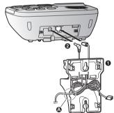
3 Insert the hooks on the wall mounting adaptor into holes (♠) and (♠) on the base unit.
