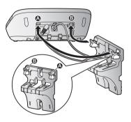
4 Adjust the adaptor to hold the base unit, then push it in the direction of the arrow until it clicks into place.
